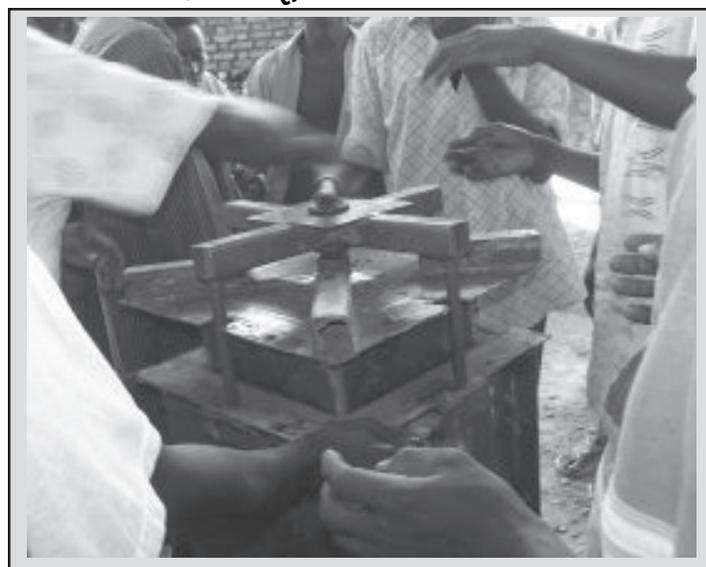
Cranking out the inside of the filter which is poured upside down and then turned over.
